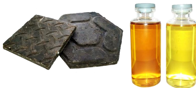
Fig.2. Paving blocks (left) from the residue of plastic waste heating and two oil fractions from heating smoke of plastic waste (right).
