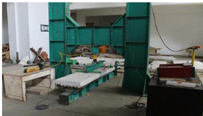
Fig.2. Flexural test setup
