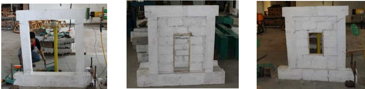
Fig. 2. Failure Pattern of F0 (left), F2 (middle) and F3 (right)
