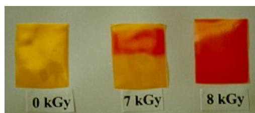
Fig. 1. PVA-CH composite films at different doses
