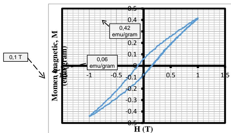
**Figure 3.** Hysteresis curve samples  $\text{BaFe}_{11,4}\text{Co}_{0,3}\text{Mn}_{0,3}\text{O}_{19}$
