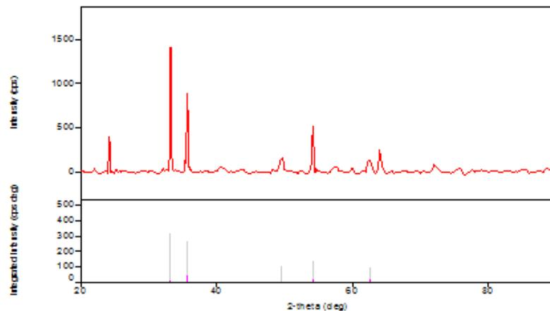
**Figure 1.** XRD diffraction patterns for material  $\text{BaFe}_{11.4}\text{Co}_{0.3}\text{Mn}_{0.3}\text{O}_{19}$  and calcination temperature of  $800\text{ }^{\circ}\text{C}$
