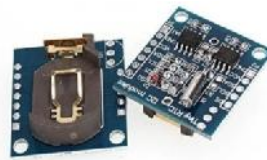
Figure 1.5 RTC module (Source: www.sfe-electronics.com )
