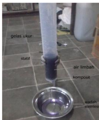
Figure1. Schematic Diagram to adsorb liquid waste
