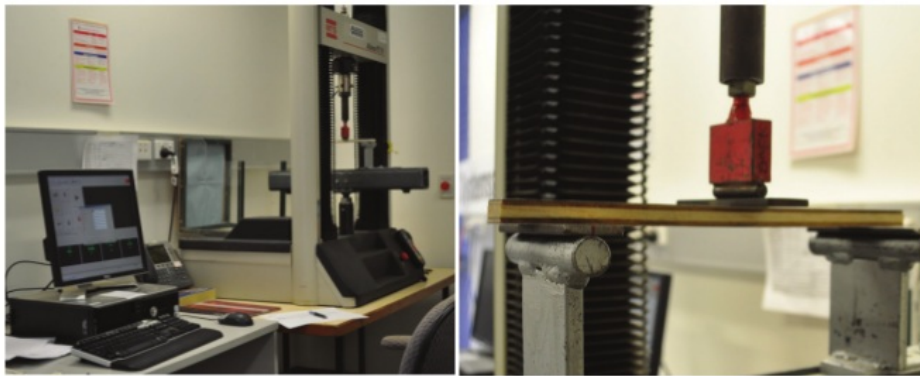
Figure 1. Test set-up for three-point-bending load
