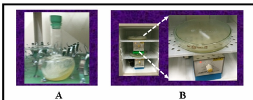
Figure 1. Bioreactor used in this study. A = conventional bioreactor (Sakaguchi flask) with shaker, B = large surface bioreactor (Petri dish) equipped with magnetic stirrer
