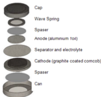
Figure 1. Design of aluminum ion battery (coin cell).
