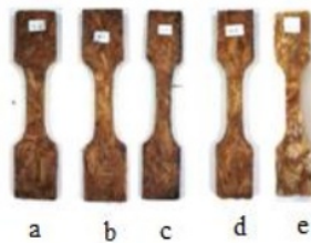
Figure 1: Composite Tensile Test Samples of Mixed Banana and Pineapple Fiber a (10: 90)%, b (20: 80)%, c (30: 70)%, d (40: 60)% and e (50: 50)%.
