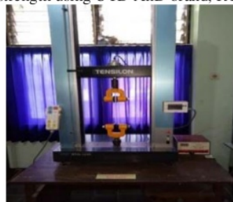
Figure 2. Tensile strength test equipment
