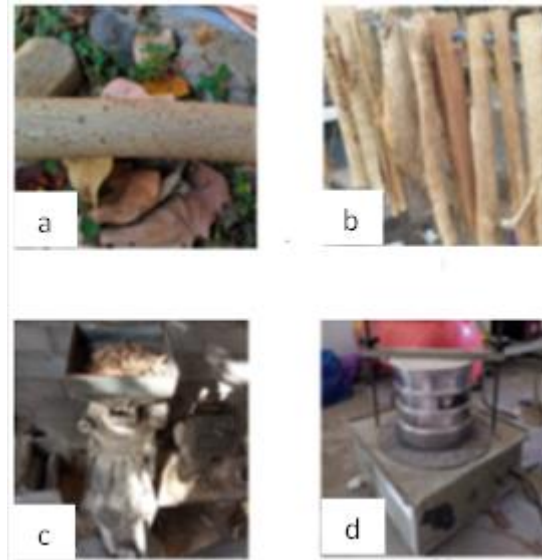
Figure 1 The making process of HTBP, a. Taking Hibiscus tiliaceust bark, b.Drying, c. Grinding, d. Screening.
