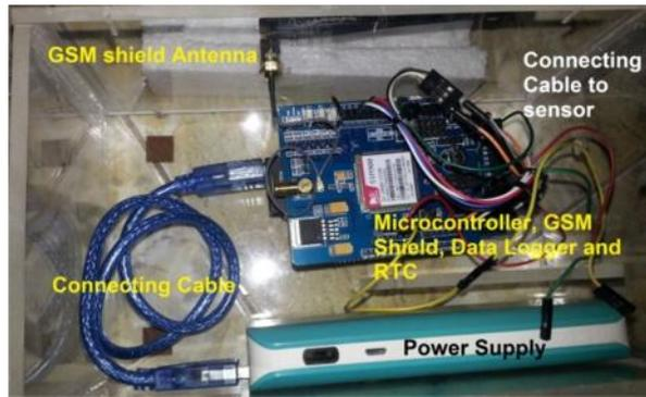
**Figure 3. A prototype of data acquisition system.**
