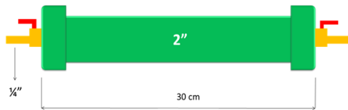
Fig. 1. The shape of the adsorber
