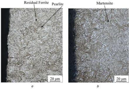
Fig. 3. Surface microstructure of the AISI 9310 steel after pack carburizing quenching (carburizing agent 70 % RHC, 30 % CESP) at 875 °C, soaking time of 3 hours: a — without vibrator quenching; b — using vibrator quenching
