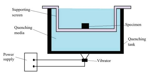
Fig. 1. Basic principle of vibrator quenching
