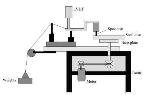
Fig. 2. Pin-on-disc wear testing machine
