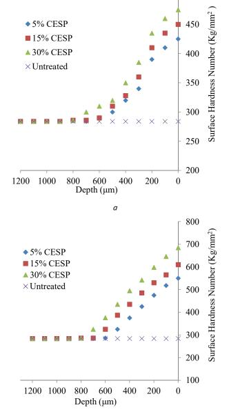
Fig. 4. Effect of carburizing agent on the surface hardness of the specimen: a — quenching without vibrator; b — quenching with vibrator
