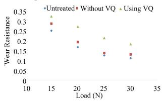
Fig. 5. Effect of vibrator quenching on the wear resistance of the specimen after pack carburizing treatment at optimum conditions
