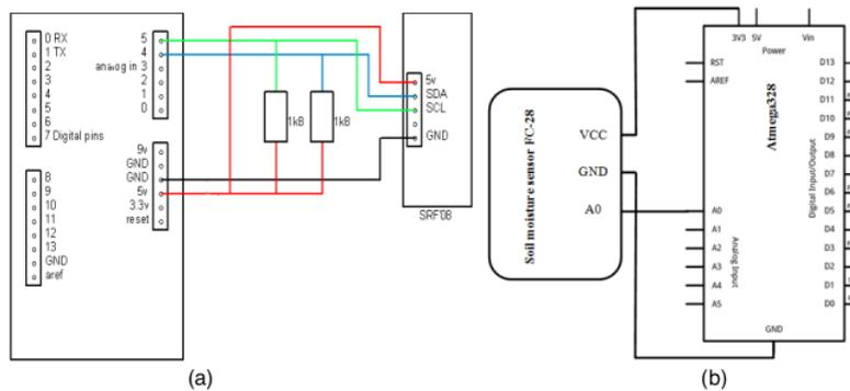
Gambar 2. Skema rangkaian: (a) sensor ultrasonik SRF08, (b) rangkaian sensor FC-28.
