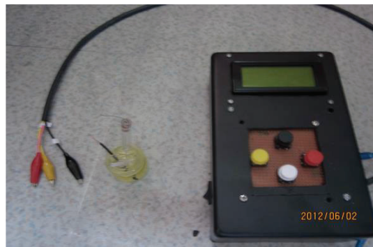
FIGURE 6. Photo of development potentiostat
