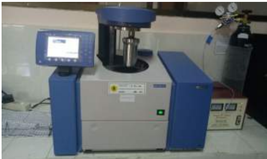
Fig. 2. Bomb calorimeter type IKA C-5000. 20
