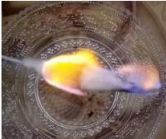
133 134 Fig. 3. MF bioethanol and premium flame test. 20
