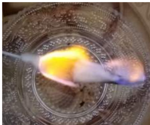
Figure 2. MF bioethanol and premium flame test.
