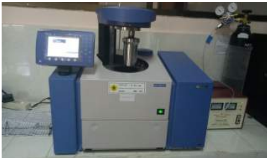
Fig. 2. Bomb calorimeter type IKA C-5000. 20
