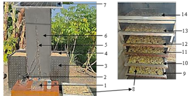
1. Data logger; 2. Cup anemometer; 3. Furnace; 4. Rice husk; 5. Thermocouple K type; 6. Drying chamber; 7. Solar panel; 8. White turmeric; 9. Shelf 1; 10. Shelf 2; 11. Shelf 3; 12. Shelf 4; 13. Shelf 5; 14. Shelf 6
