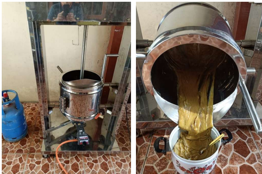
Figure 2 Fruit lunkhead stirrer machine
