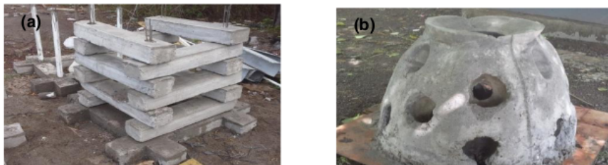
Fig. 8. The armour block of model, a) the OCB, b) the Reefball.
