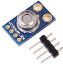
Gambar 2 sensor suhu MLX90614
