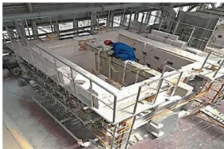
Fig. 3. Beam specimen fire test set-up
