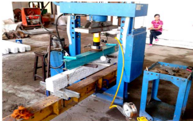
Fig.3 Flexural Testing Set-up of the Beam
