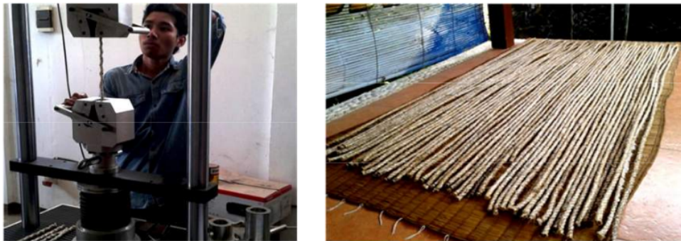
Fig. 1 Sisal Specimen under Tensile Test (left) and Bars Reinforcement of Sisal Fibres (right)
