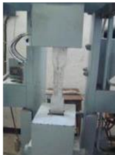
Fig. 1 Tensile testing of cold-formed steel
