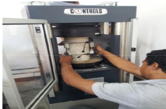
Figure 5. Set-up Compression and Modulus of Elasticity Test
