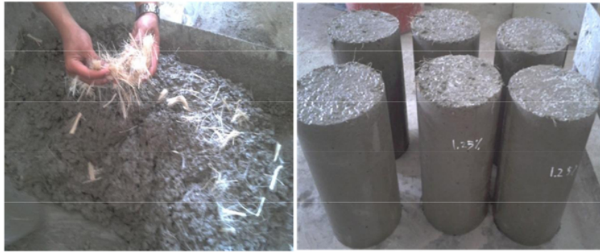
Figure 4. Fibrous Concrete Specimen Preparation
