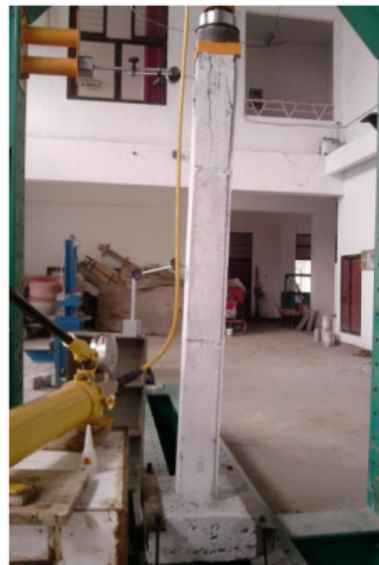
Figure 5. Set-up column under axial load.
