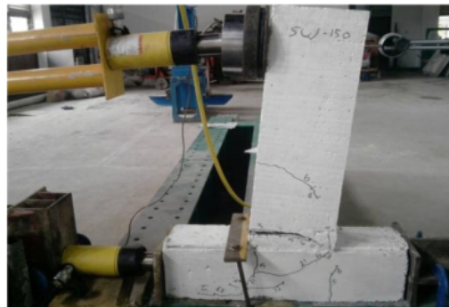
Figure 7. Typical beam-column joint test.
