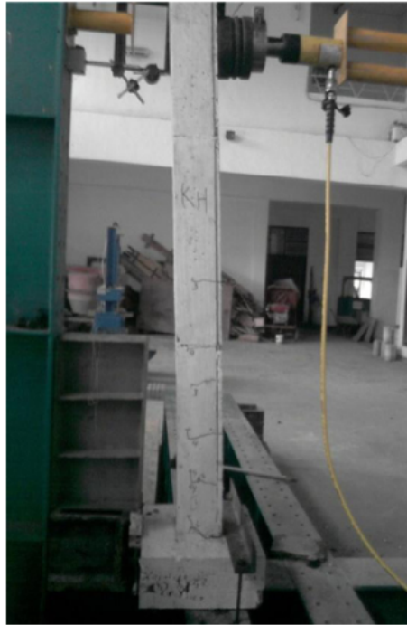
Figure 6. Set-up column under lateral load.
