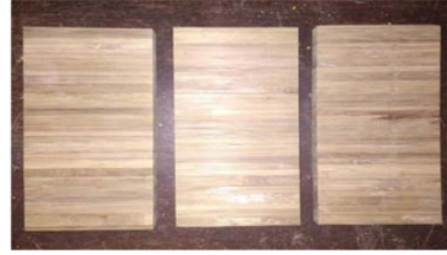
Fig.3 Specimens creep shear test of glued-laminated bamboo
