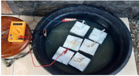
Gambar 6. Proses Pemberian Initial Corrosion
