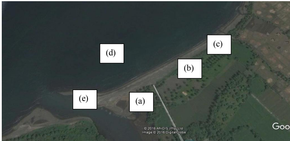
Figure 2. Site analysis based on topography. (a) Empty land that can be used for parking lots. (b) Empty land that can be used to support coastal tourism, namely culinary (restaurant). (c) Empty land that can be used for green open space. (d) The effect of the direction of the ocean waves that can collect sand on the beach, can be directed to make Jetty for fishing. (e) Boat mooring is developed into a quay with supporting facilities.
