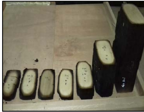
Figure 5. Charring depth at some positions.
