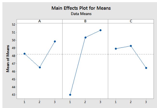
Fig. 1. Main Effect Plot Mean of Mortar Compressive Strength
