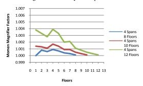
From the above results, it can be seen after conducting a P-Delta analysis of the structure that is reviewed with varying spans and heights to obtain the amplification factor, the final moment, and deflection due to the P-Delta effect. The deflection value and the last moment are more significant than the first moment, so it needs to be controlled against the deflection, and the moment that occurs.
