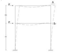
Picture. Story Drift and Drift on the portal
