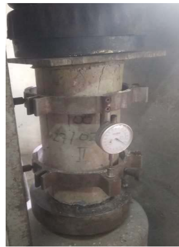
b. Compressive testing
