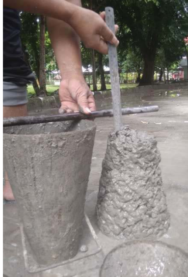
FIGURE 3. Fresh properties of testing concrete
