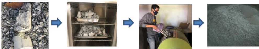
FIGURE 1. Waste concrete generation during recycled aggregate production
