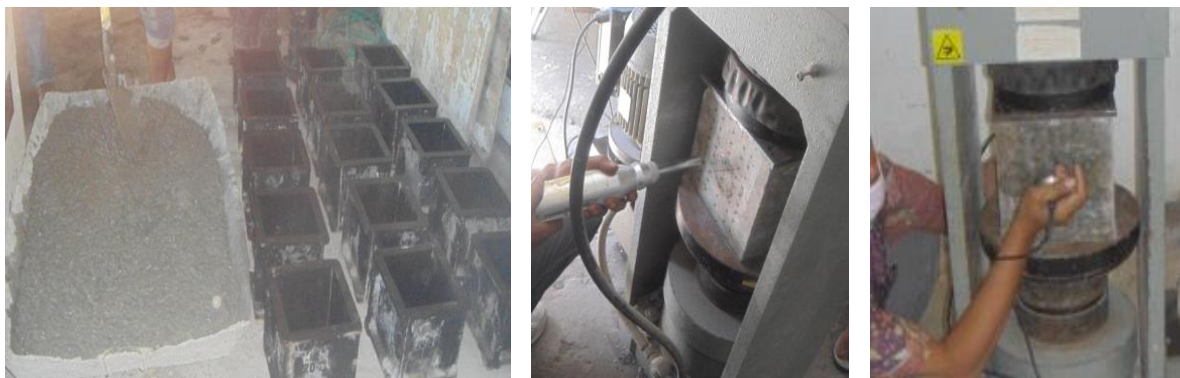
Figure 1. Concrete casting and testing
