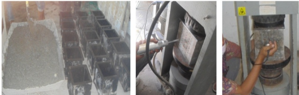
Figure 1. Concrete casting and testing
