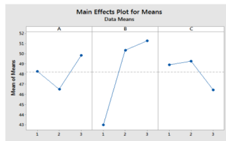
Figure 1. Main effect plot mean of mortar compressive strength for factor A, B, C
