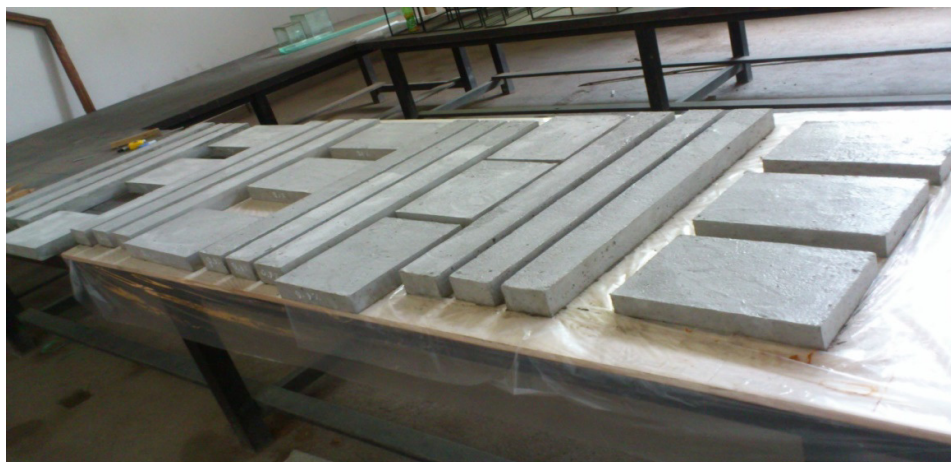
Figure 4. Specimens treatment in high temperature and low humidity room
