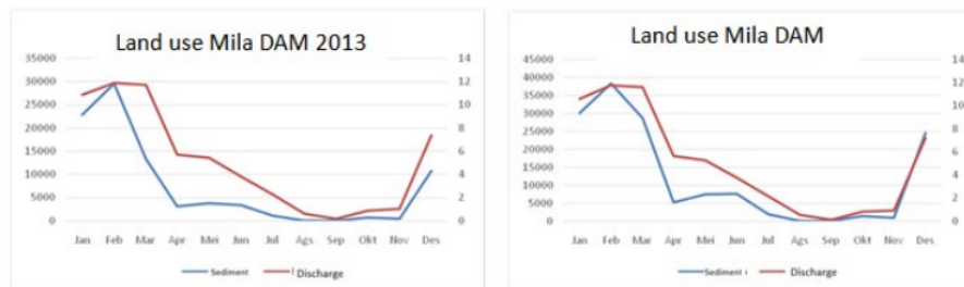
Figure5.(a) Graph of Correlation between Sediment Transport and Mila Dam Discharge with Land Use in 2013 (left), and (b) Graph of Relationship of Sediment Transportation with Mila Dam Discharge with 2018 Land Use (right)
