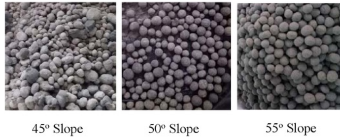
Fig 5. Artificial aggregates with \text{Na}_2\text{SiO}_3/\text{NaOH} ratio of 2.5 and slope variations [11]
