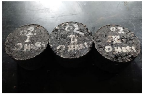
Figure 2: Specimens of compaction of asphalt-concrete mixture
