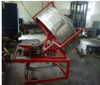
Fig. 2. Granulator for aggregate manufacture
