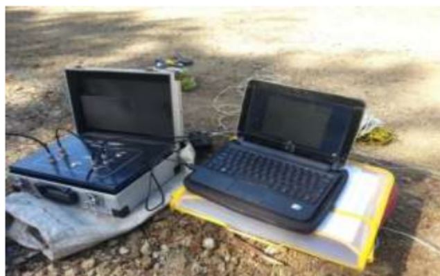
Gambar 3. Multi Channel Resistivity merk S-Field
