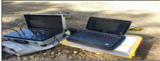
Gambar 3. Multi Channel Resistivity merk S-Field
