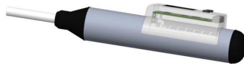
Figure 4. The schematic view of intelligent rebound hammer.
