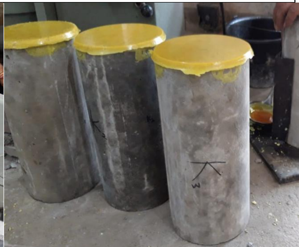
Proses capping beton
