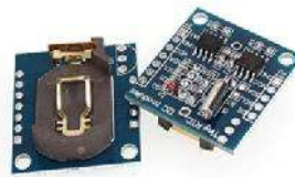
Figure 1.5 RTC module (Source: www.sfe-electronics.com )
