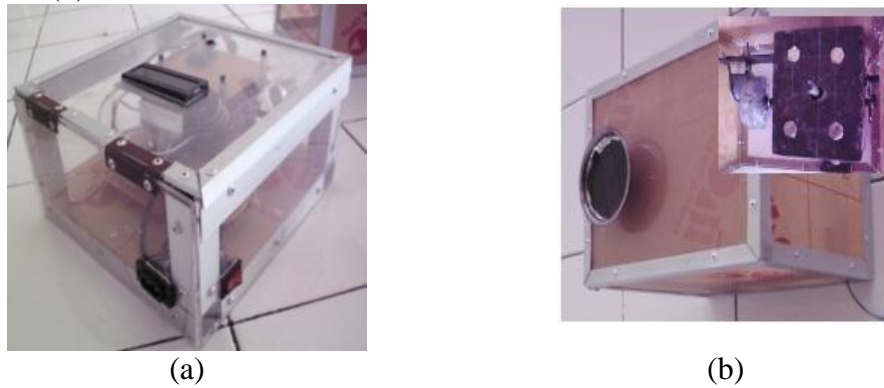
Figure 3. Low-frequency vibration generators.
