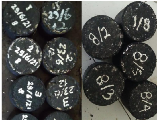
(a) Hot compacted (b) Cold compacted
