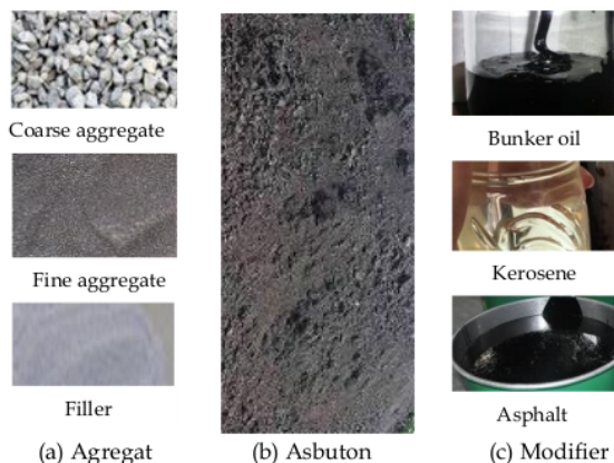
Figure 1. Asphalt mixture material
