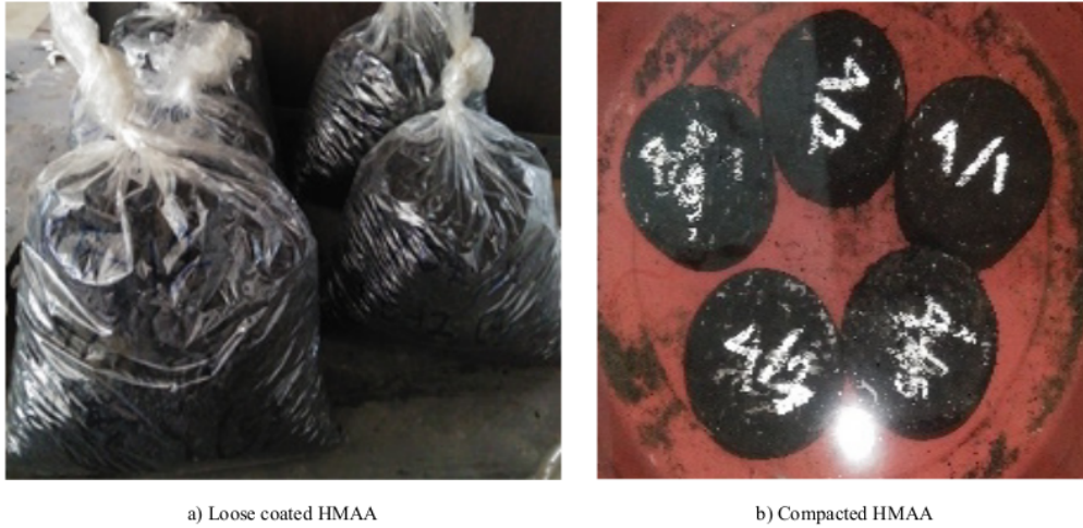
Figure 7. Asbuton mixture and specimens in the curing process
